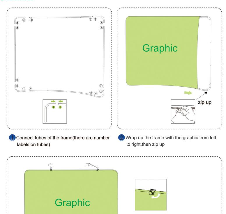
Put the light clip on the top of display and fix it with screw, then connect the light and the clip
